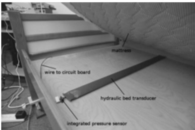
Fig. 1. Positioning of bed sensor for testing
