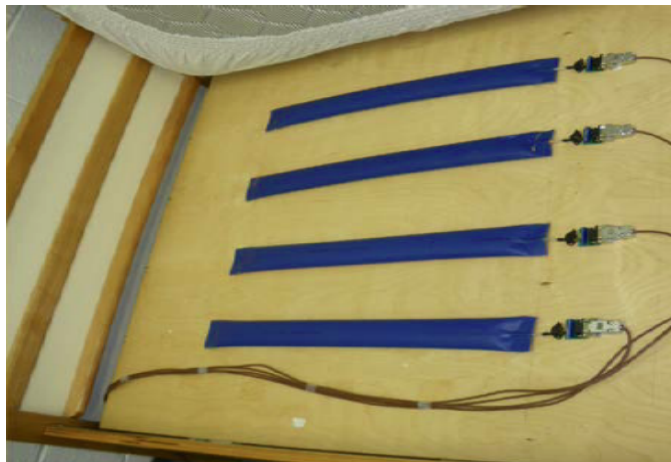
Figure 1. Hydraulic bed sensor multi-transducer configuration.
