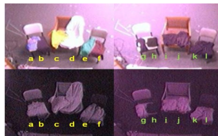
Fig. 4. The cloth color in visible and IR light condition; the images in the top row are collected in visible-light-condition; the images in the bottom row are collected in IR-light-condition; The fiber types are listed in TABLE I. The cloth h in IR light condition is dark because of its low areal density.
