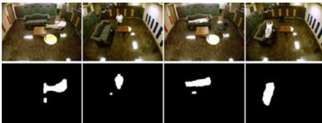
Fig. 6. Example images and their corresponding silhouettes from the fall data set. Lying on the couch and sitting on the chair with feet up activities, which could be misinterpreted as a fall, are not recognized as a fall in our system, an advantage of rule-based reasoning and knowledge about three-dimensional voxel person.
