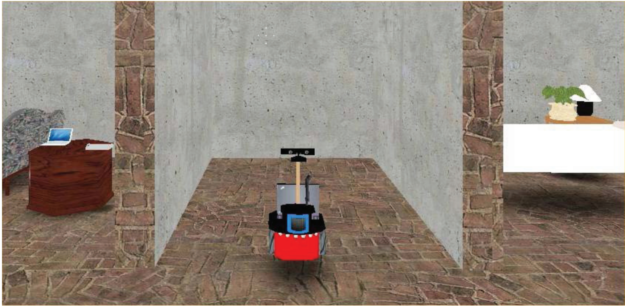
Fig. 1. The virtual scene used for the human subject experiments, showing the robot avatar in the hallway with the living room on the left and the bedroom on the right. The robot and virtual environment are modeled on the physical robot and environment in which future experiments will be conducted. The Microsoft Kinect will be used for perception on the robot.
