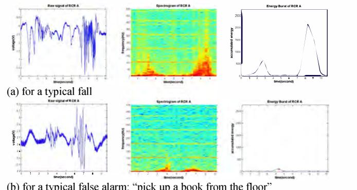
Fig. 3. Doppler signal (speed), spectrogram and energy burst captured by RCR sensor A
