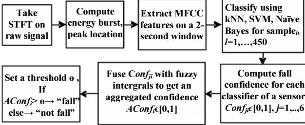
Fig. 2. The flowchart of fall detection algorithm
