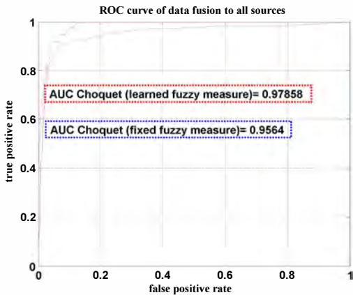
Fig. 5. Data fusion with Choquet integral (a) blue dot curve is from with fixed fuzzy measure from information sources' AUC; (b) red dash curve is with learned fuzzy measure.
