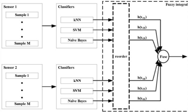
Fig. 1. The diagram of a fall detection system with fuzzy integral fusion
