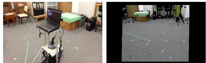
Fig. 5 The left image is a scene photo taken by an external camera. The right image show a view from robot Kinect camera.
