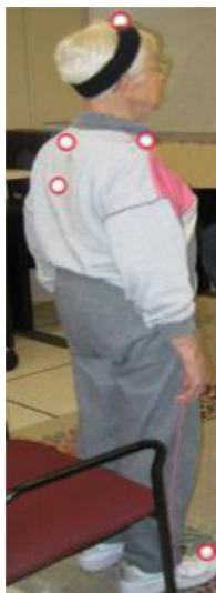
Fig. 7. Elderly participant with markers on the head, shoulder, two on the back and feet (highlighted in red) for the VICON motion capture system.
