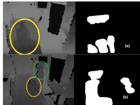
Figure 4. The depth image and corresponding horizontal surfaces obtained after removing the ground plane. In Figure 4 (a), there is a patient lying in the bed circled in yellow and in Figure 4 (b), there is a patient and hospital staff member, circled in yellow and green respectively.
