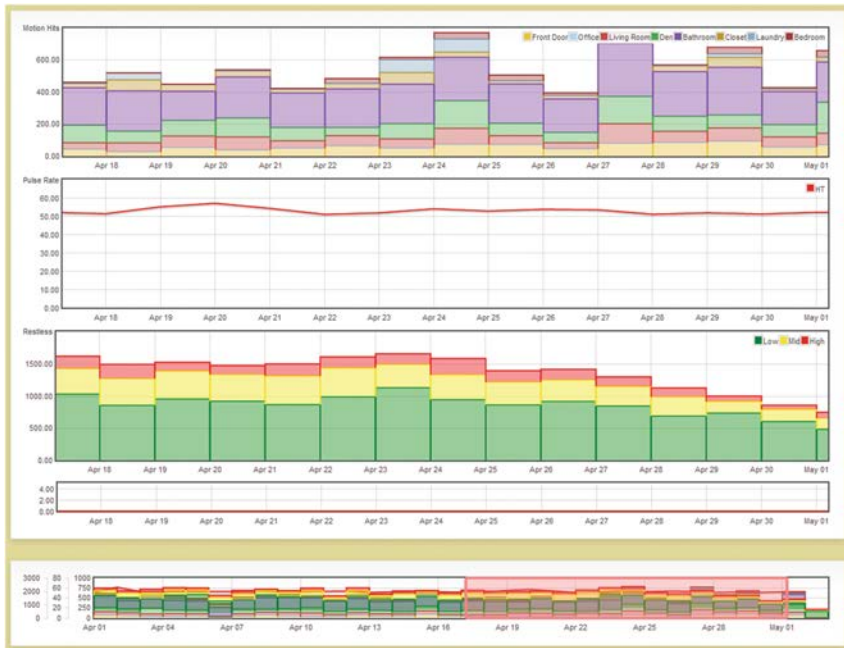
Fig. 2. View of sensor data on the improved Version 2 interface showing motion data (row 1) pulse rate (row 2), and bed restlessness (row 3). Notice the time range selection bar at the bottom (row 4). The highlighted date range is the range displayed in the large view.
