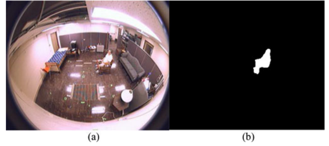
Fig. 2. (a) RGB image of the side profile of a person sitting on the chair. (b) Silhouette extracted after extracting the foreground from the image.
