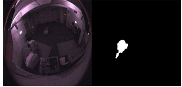
Fig. 6. Silhouette quality obtained using IR emitters in a dark room. This shows a stark difference with the silhouette obtained in Fig. 2.
