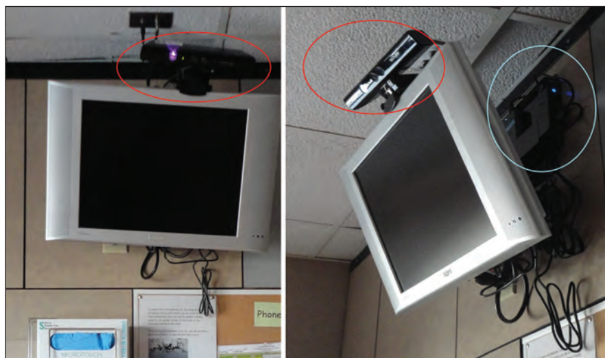
Figure 2. Front and side view of a Microsoft® Kinect™ sensor (circled in red) mounted above the television in a hospital room. The EEEBox computer along with the external hard drive is circled in blue.
