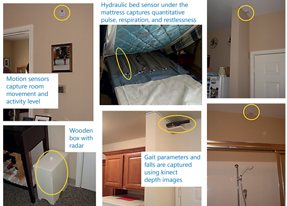
Fig. 2. Sensors in the living environment.
