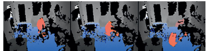
Fig. 5. Depth images of a TigerPlace resident fall detected by Kinect.
