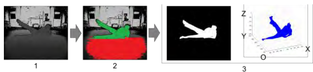
Fig. 2. Preprocessing steps: 1) Raw depth image; 2) Extract floor plane and pixels in game region; 3) Extract player and transform points to floor coordinate reference
